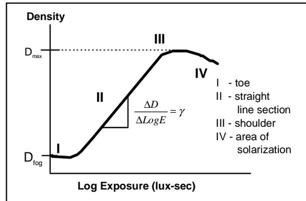
Figure 2 - A Typical Characteristic Curve
