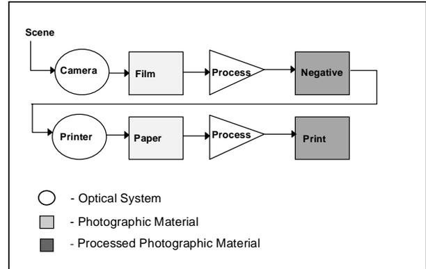
Figure 1 - Block diagram of the print photography process
